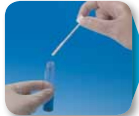
Attach the strips to the cap and recap the vial
